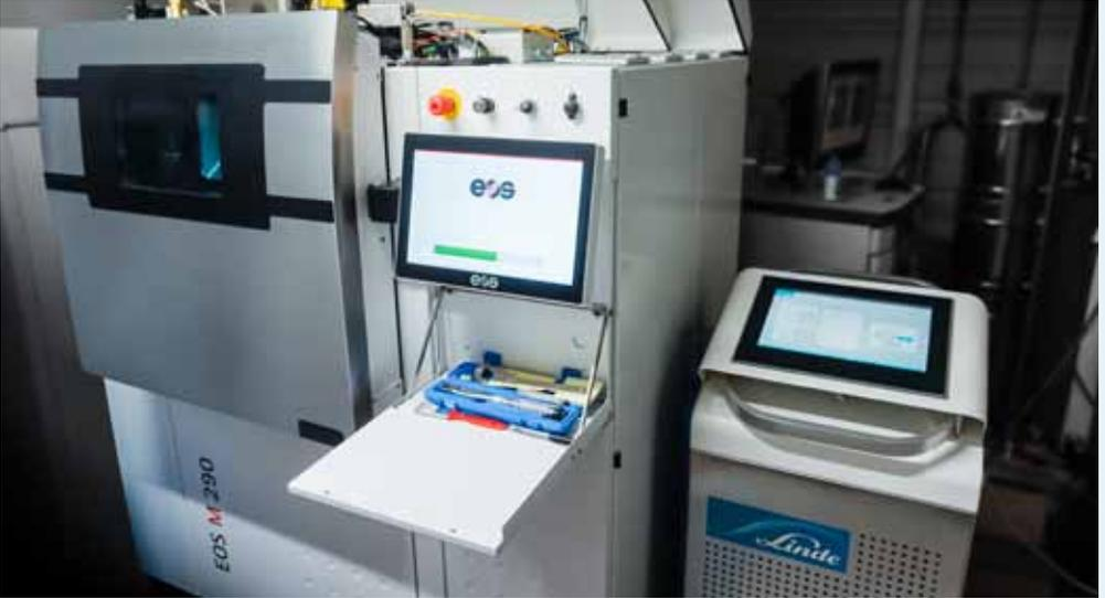
The ADDvance® O<sub>2</sub> precision solution working alongside 3D Medlab's printer.
