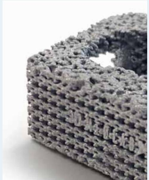
Interbody fusion cage made from Ti-6Al-4V.
